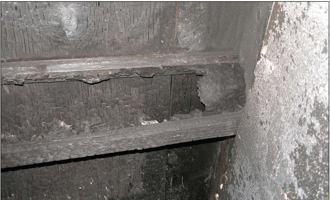
Figure 17: Test 4, first unsprinklered test, one of the few remaining engineered joists on the ceiling. Note how the webbing is almost entirely consumed.
