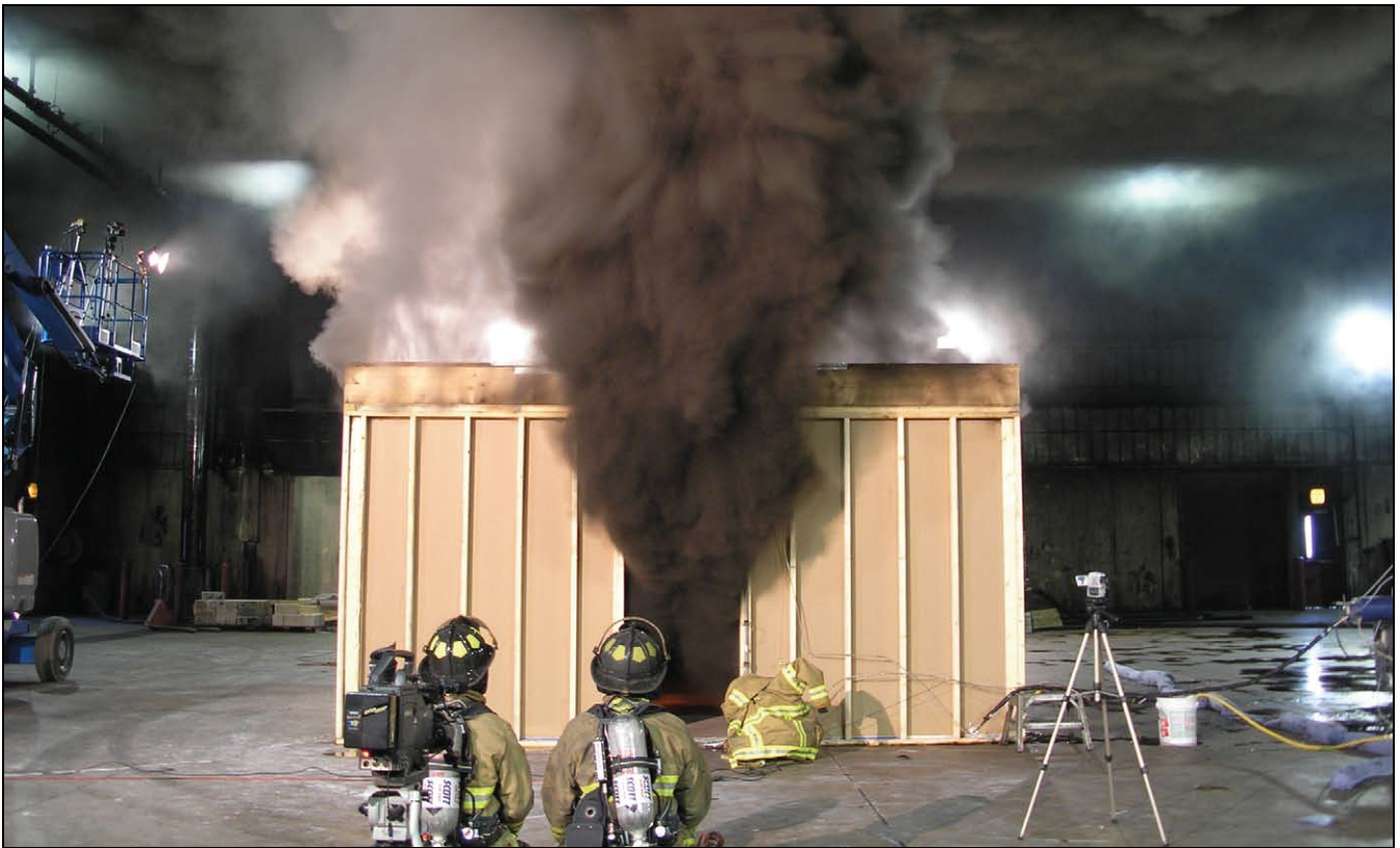
Figure 13: Test 4, first unsprinklered test, just before flashover
