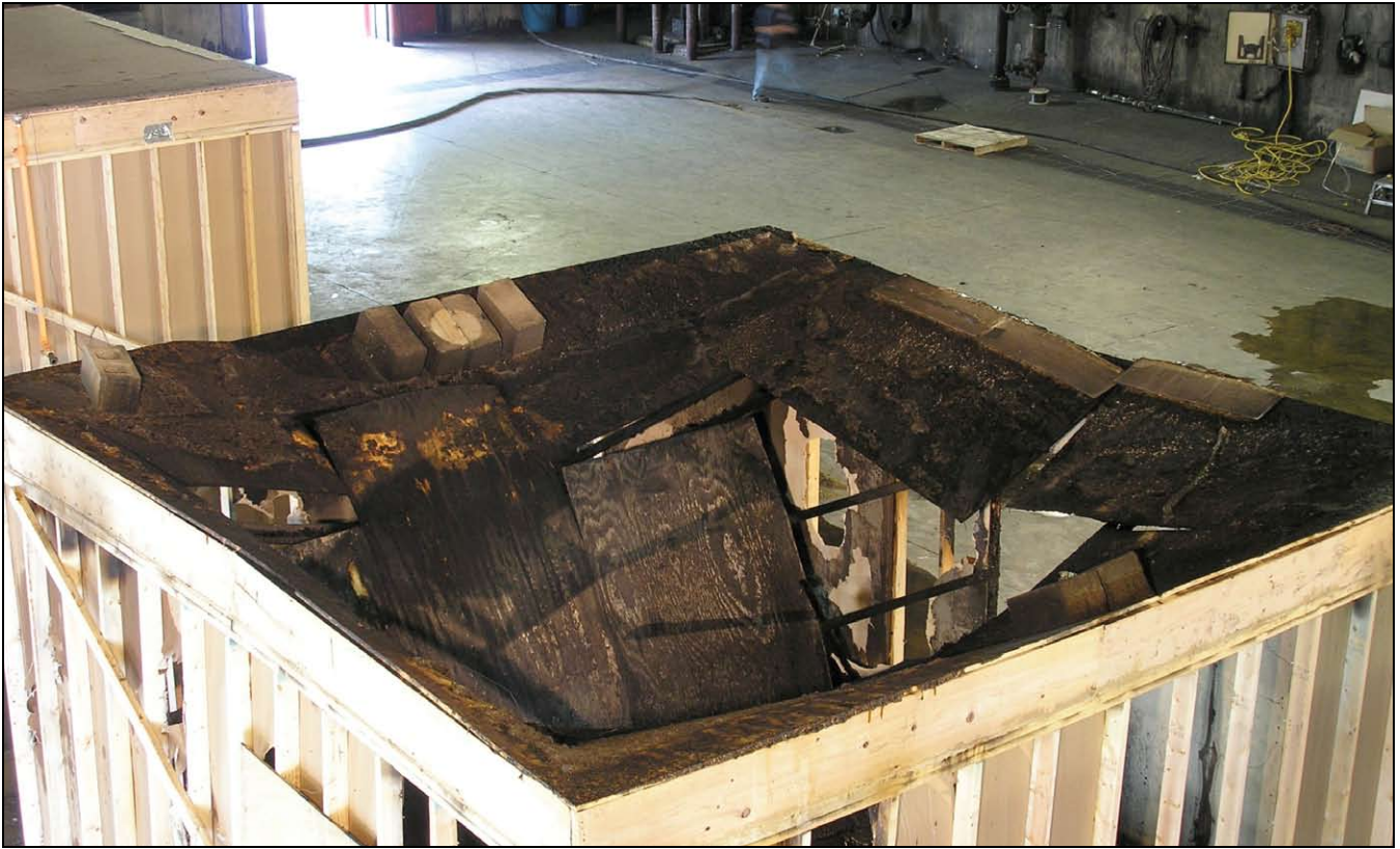
Figure 16: Test 4, first unsprinklered test, roof collapse of structure
