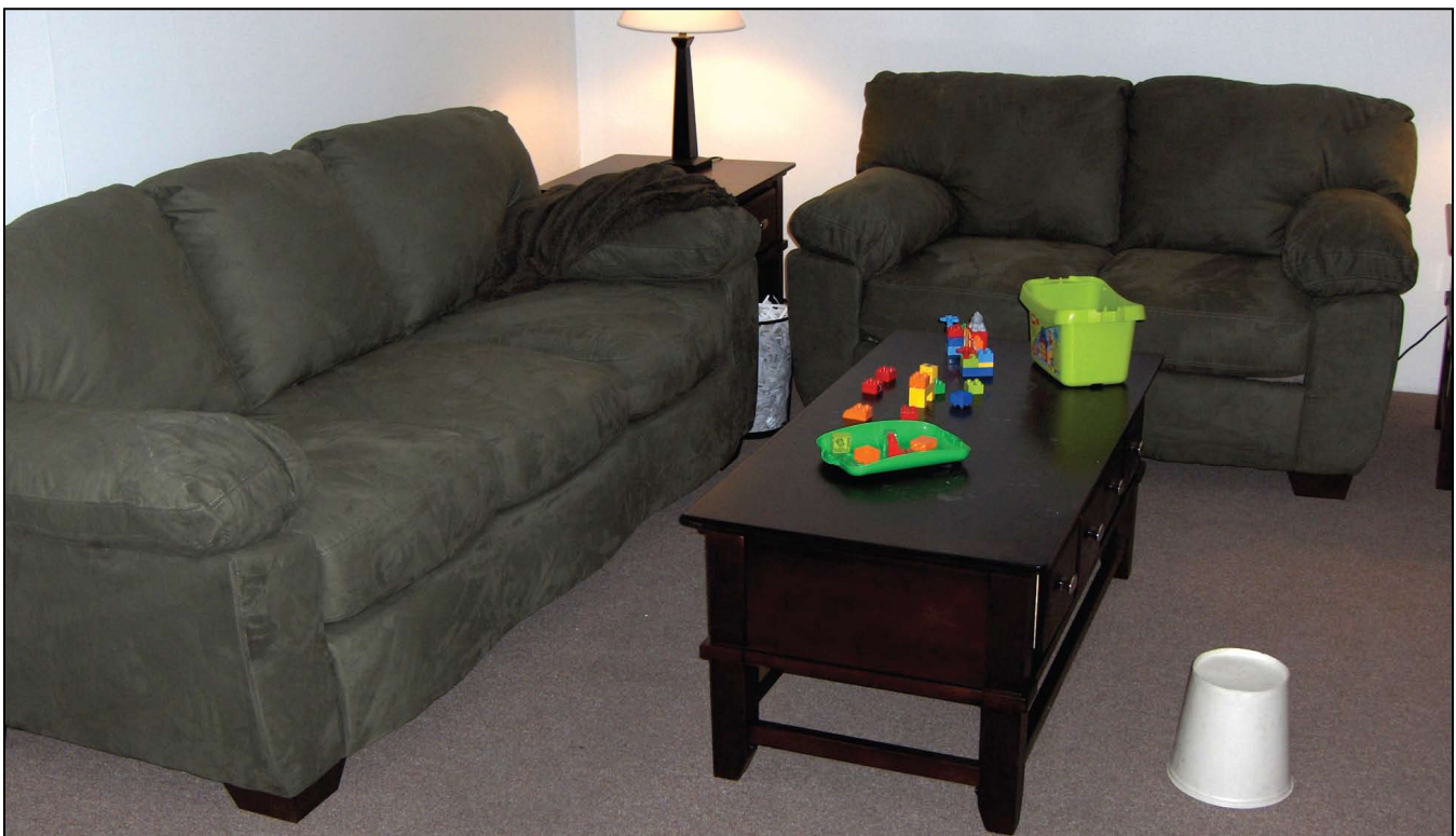
Figure 2: Fuel package used for all tests. White bucket on floor was used to protect floor radiometer during setup; the bucket was removed prior to each test.
