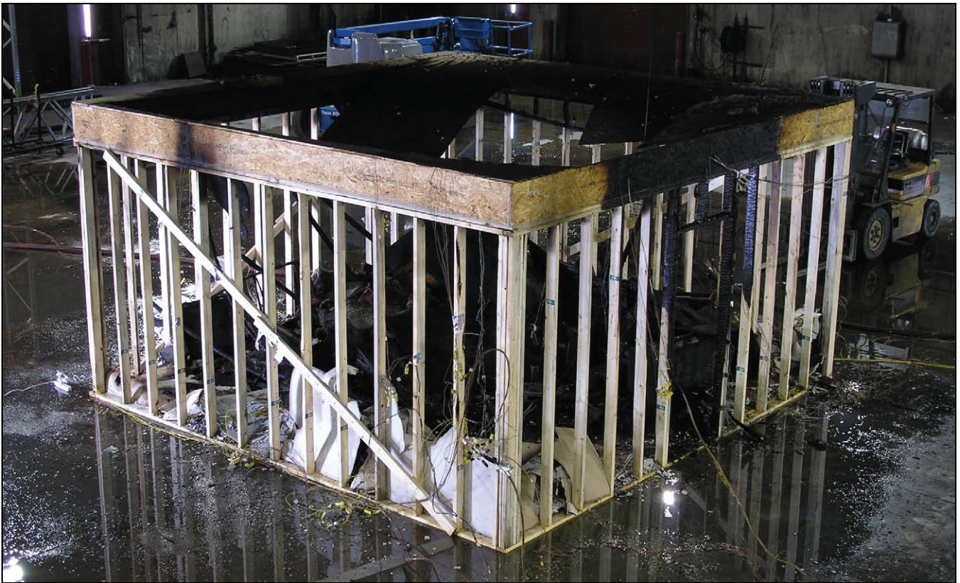
Figure 19: Test 5, second freeburn, damage
