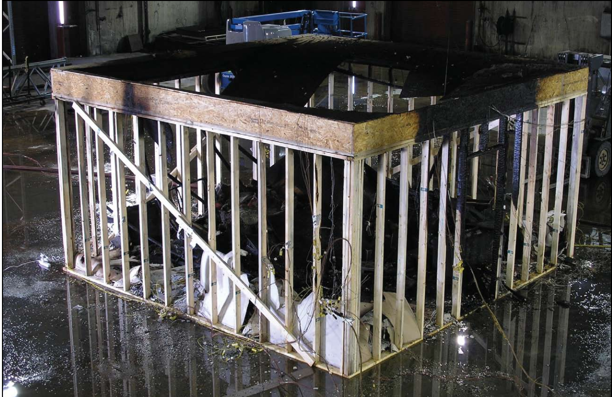
Test 5 second freeburn, damage
