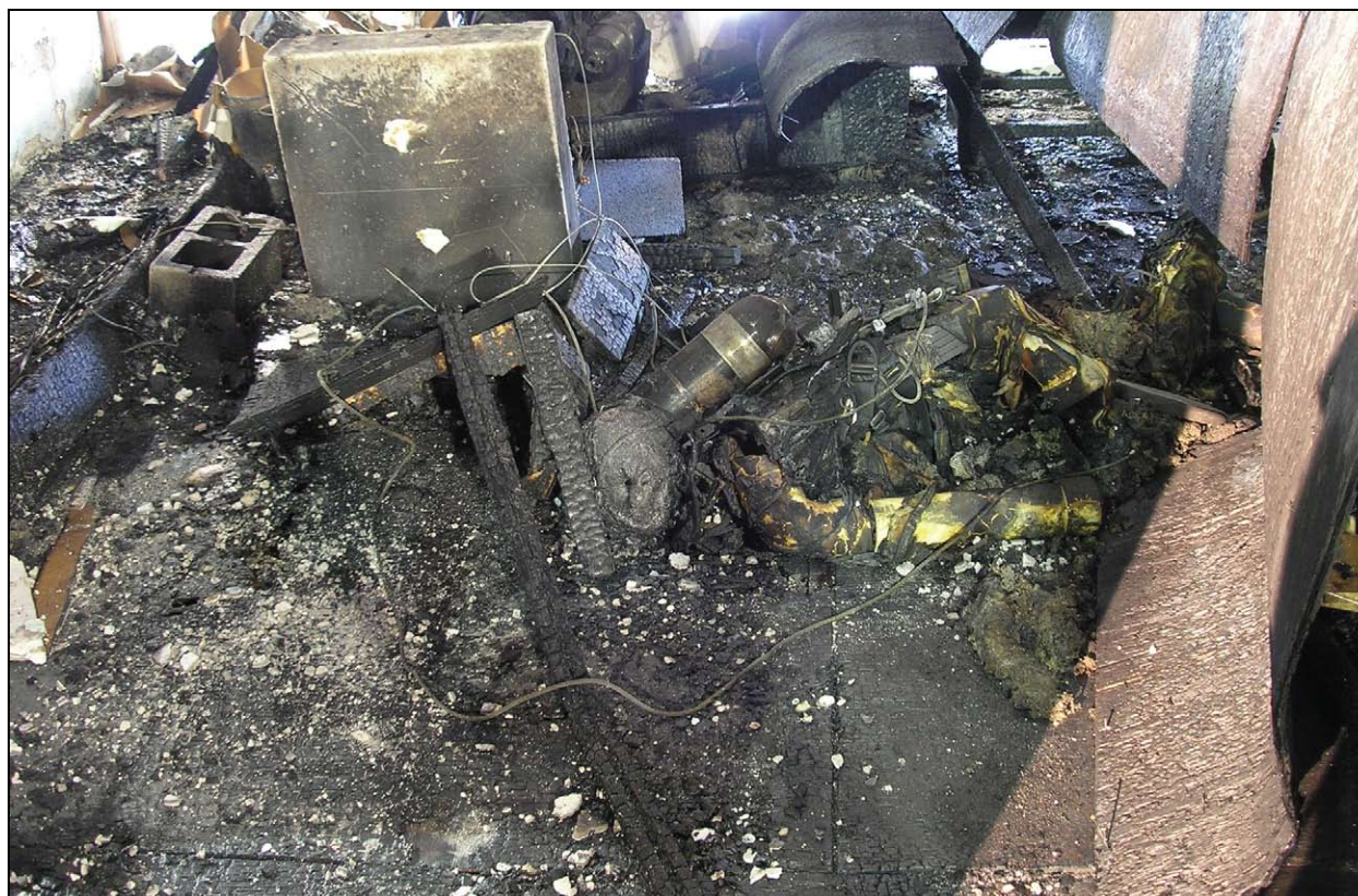
Test 4 First Unsprinklered Test, Damage
