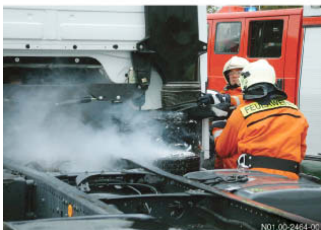
Blowing CO 2 into the air intake
