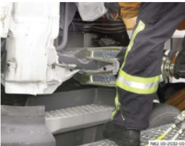
Crushing the rocker panel
