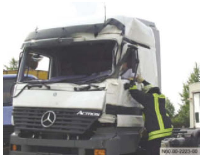
Opening doors by hand or with small tools
