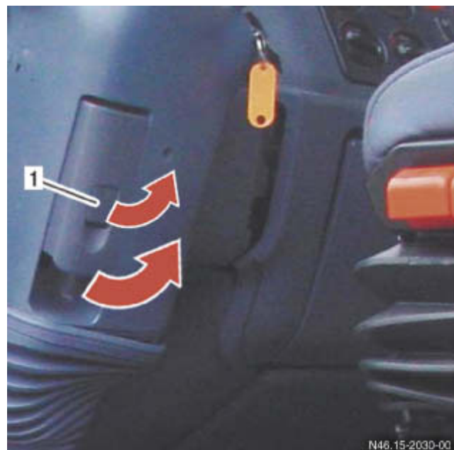
Manual release with locking mechanism
