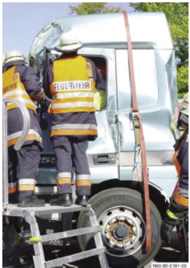
Strap around frame and cab
