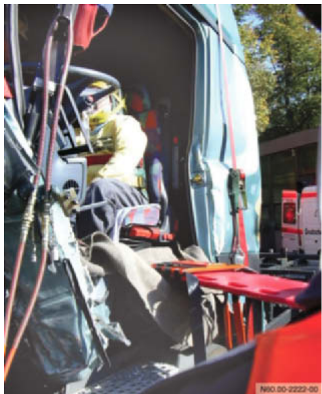
Rescue opening via the driver door
