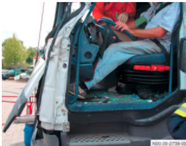
Deformed footwell (Rescue exercise at Ludwigshafen on 15.09.2001)
