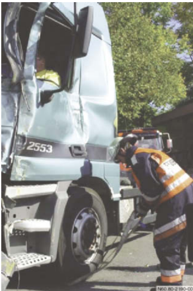
Strap around frame and cab
