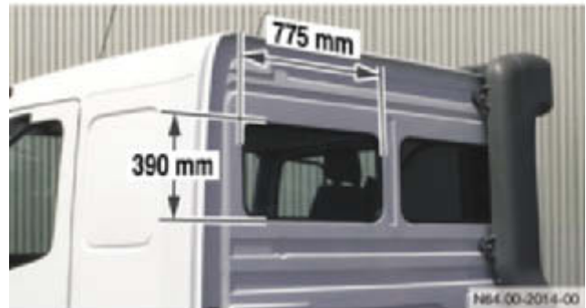
Potential access via rear window
