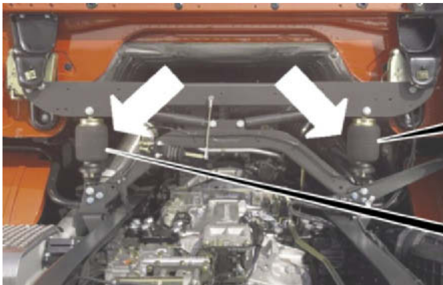
Cab mounting air bellows (1)
