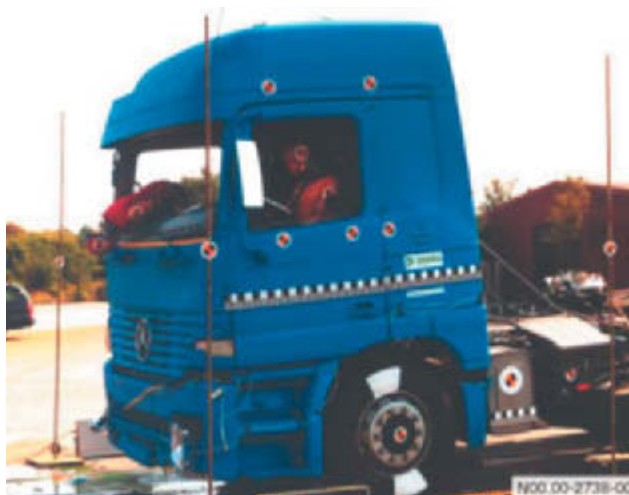
Driver strapped in, front passenger not strapped in. Collision with dummy flatbed at 30 km/h
