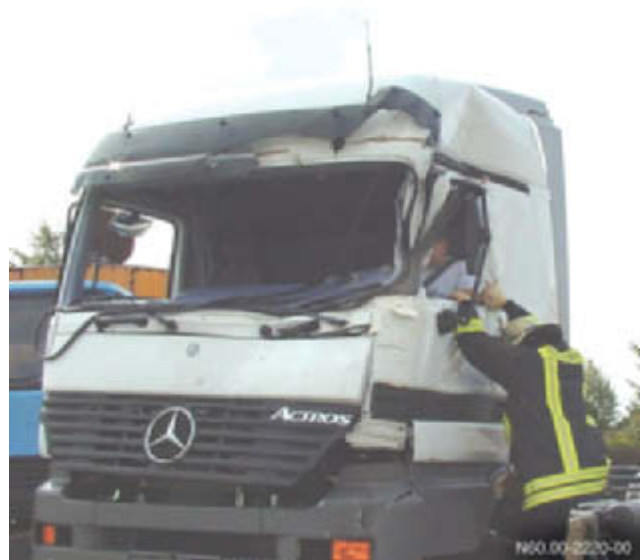
Initial assessment, e.g. through the side windows or the windshield
