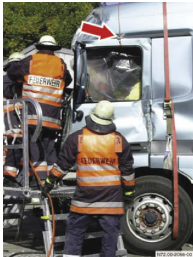
Securing the door with a rope
