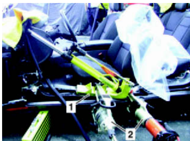
1 Sill attachment 2 Spreader
