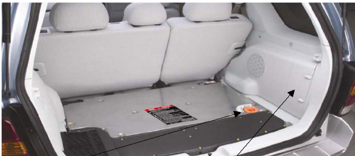
High voltage Service Disconnect Switch
