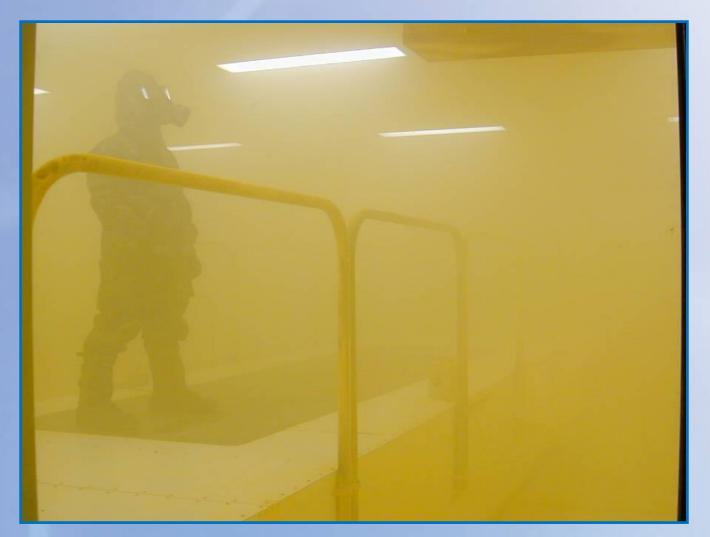
25' x 50' 10 mph ~ 70° F ~ 50% RH ~ 170 mg/m<sup>3</sup> 2.5 µm MMD
