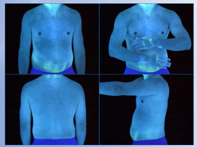
The lower front torso showed moderate to heavy aerosol deposits, and the location and pattern suggest infiltration through the coat-trouser interface. The bright spots on the hands and wrists could have been due to aerosol penetration, an artifact from doffing, or a combination of both.
