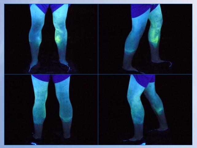
The lower legs had a high level of deposited aerosol. The patterns suggest aerosol infiltration through the boot-trouser interface and possible penetration through the trouser fabric.
