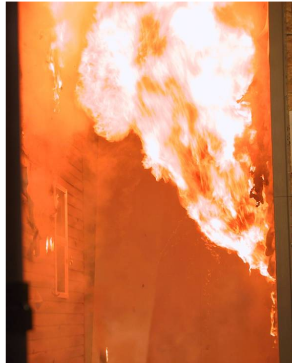
Unrestricted Construction Experiment: Target Wall OSB Ignited 1 min 20 sec. after Window Failure
