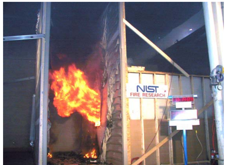
Fire Resistant Construction Experiment: 9 Minutes after Window Failure – Target Wall OSB not Ignited
