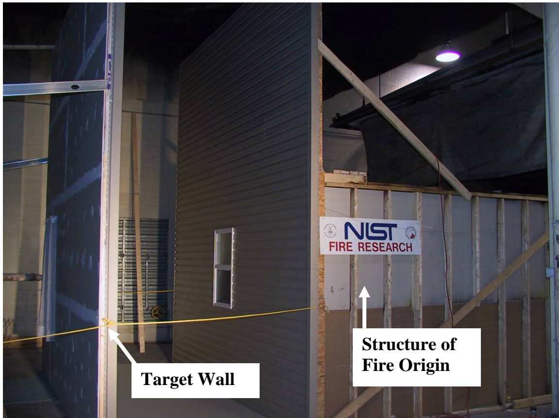
Structure of Fire Origin and Target Wall
