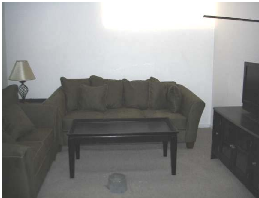
Figure 4-1: Photograph of the furnished living room interior. Note the gas and particle sampling probe extending into the right side of the room at standing face level.
