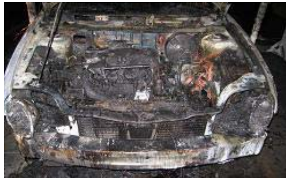
Engine compartment (post fire)
