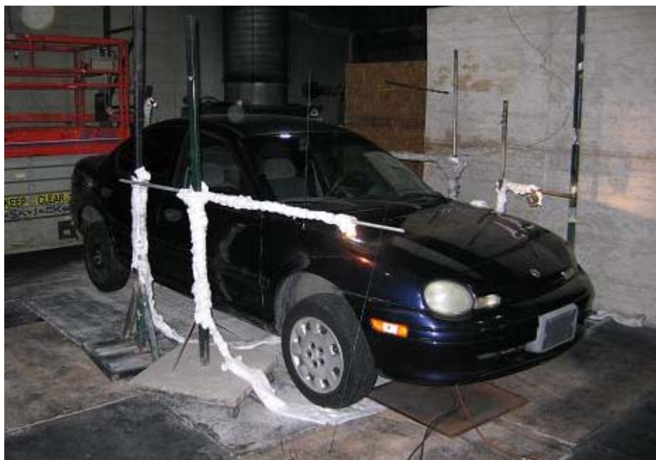
Figure 4-13: Photograph showing the automobile for the engine compartment scenario
