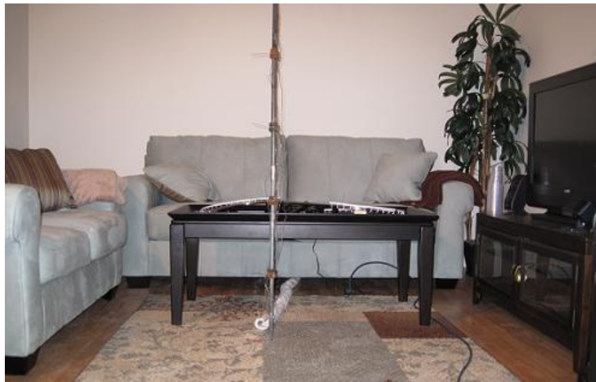
Figure 4-3: Photograph of the furnished living room interior for the limited ventilation fire test. Note the thermocouple instrumented post in the center of the room.
