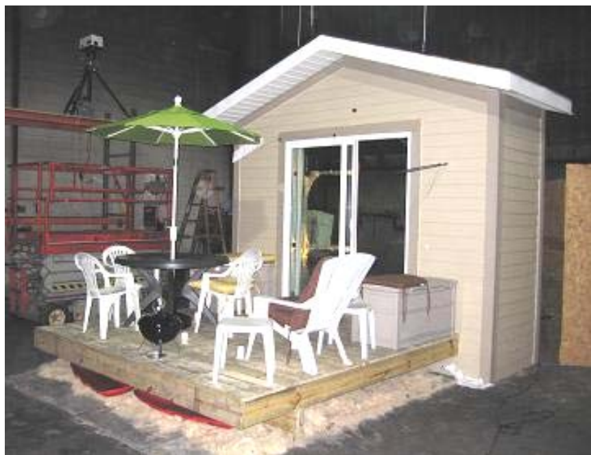
Figure 4-8: Photograph showing the wood deck scenario with furnishings. Note the the gas and particle sampling probe extending from the right of the sliding glass door over the deck at standing face level.
