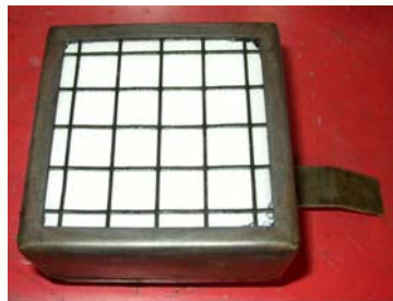
Figure 3-3: ASTM E1354 Cone calorimeter sample holder
