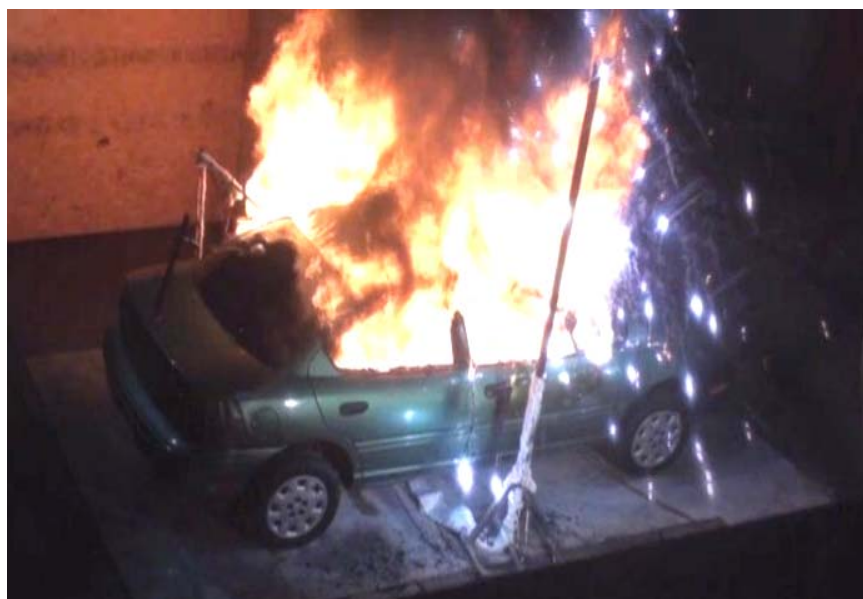
Figure 4-71: Scintillating shrapnel resulting from air bag deployment during the passenger compartment fire.
