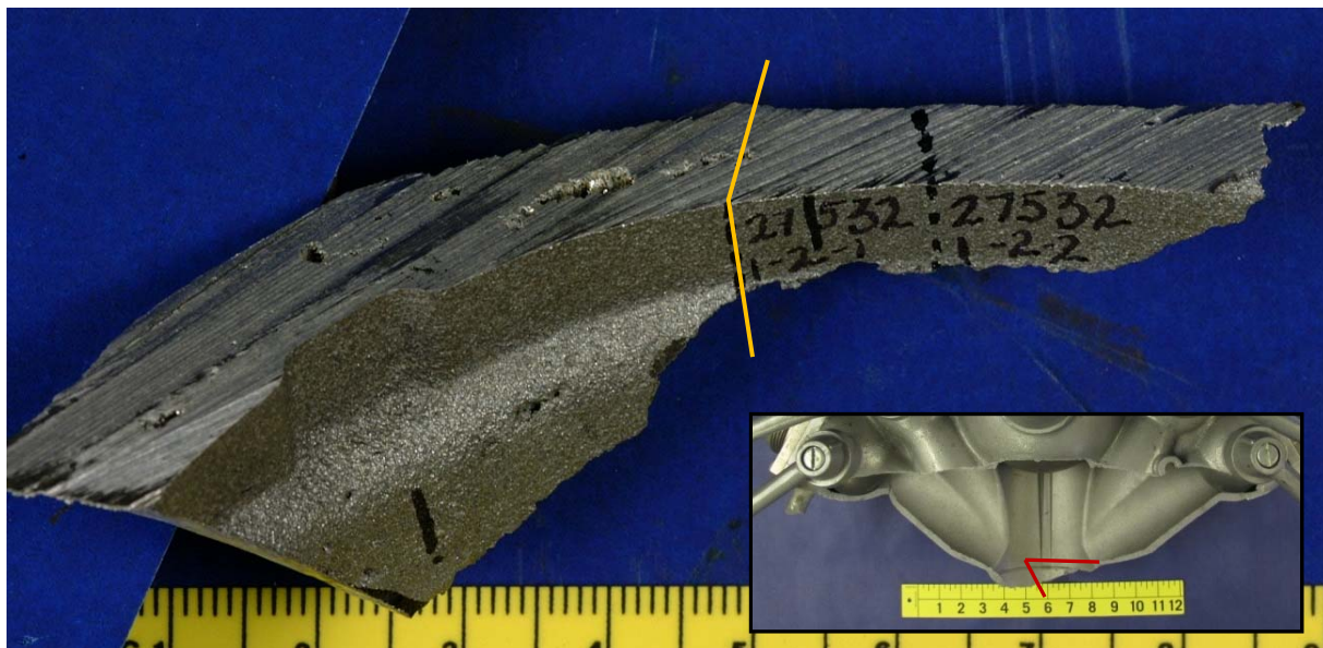
Figure 9. Cut piece from larger manifold piece showing large voids on the cut surface. Inset shows location of piece. Yellow lines show location of additional cut for cross-sectional metallurgical mount.
