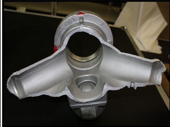
Figure 3 - Upper portion of the manifold after the failure. This is the section that struck FF Crawford (piece is lying upside down).
