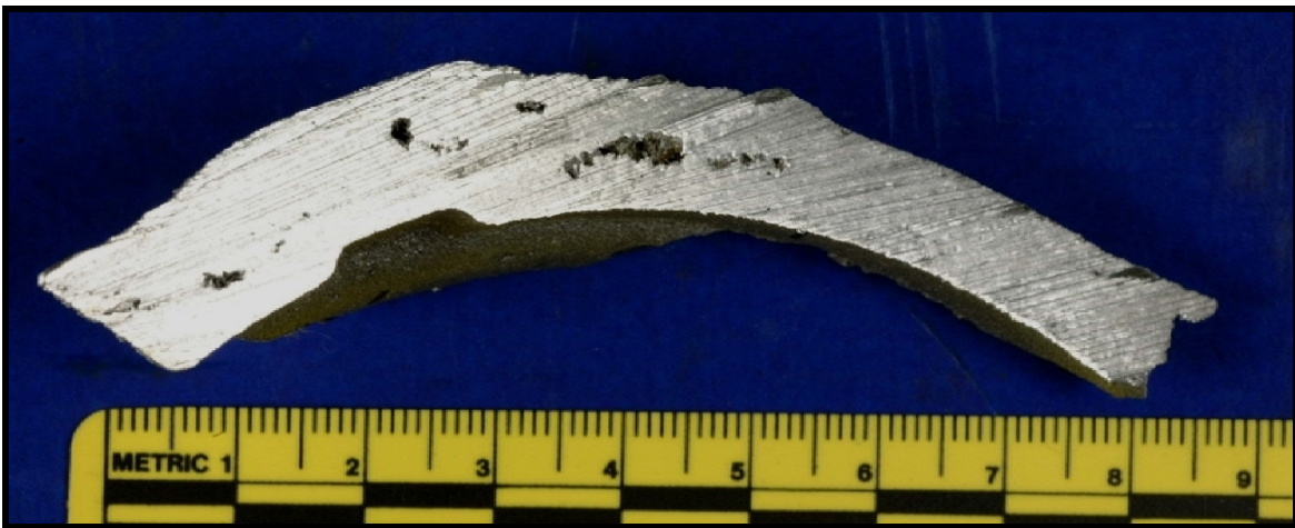
Figure 4 - Note the large voids in the cut surface of the casting wall.
