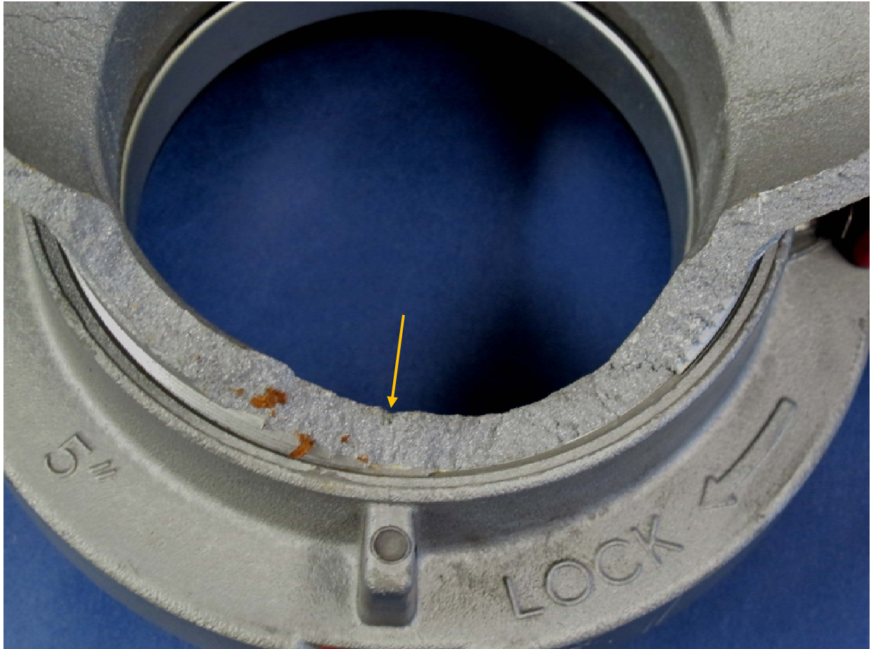
Figure 6. Closer view of fracture surface at inlet connection threads. Arrow shows location of Figures 7 and 8.
