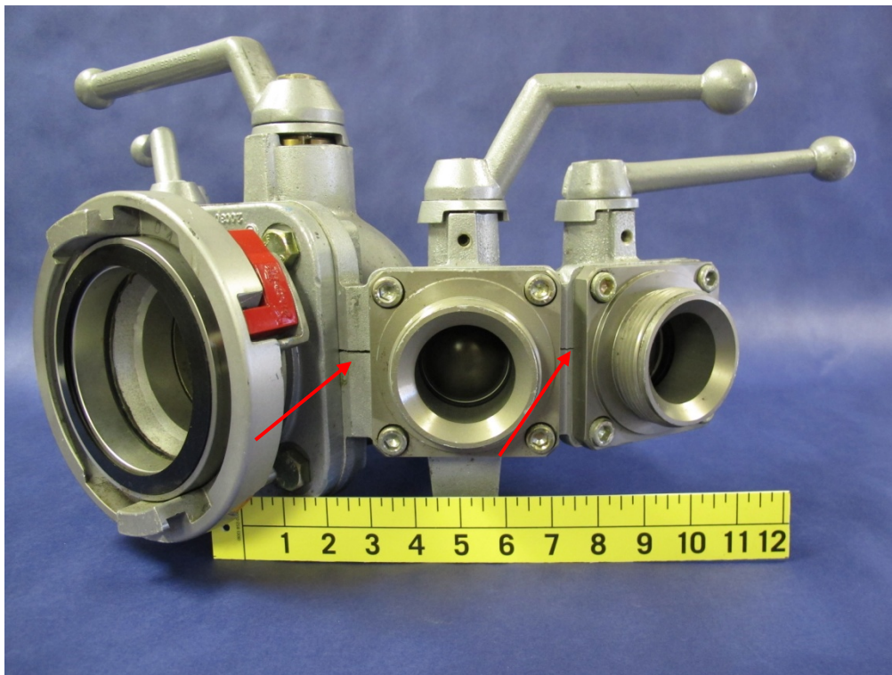
Figure 4. Additional views of the large manifold piece, showing cracking through the approximate center line (arrows).
