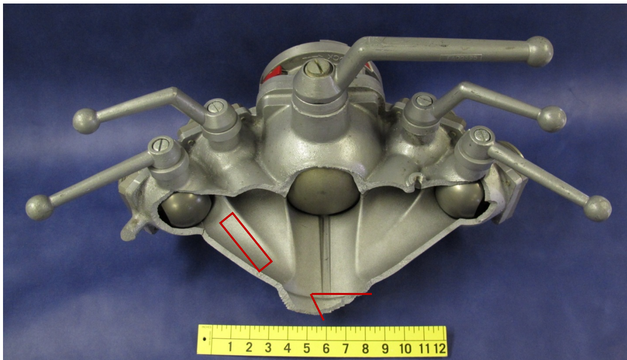
Figure 2. Two views of the larger piece. In addition to cracking that caused one piece to break away, cracking occurred all around the piece, especially through the approximate center-line of the cast manifold. The red lines on the bottom photograph show the approximate locations of cuts to remove the fracture surface for further examination, including a cross-sectional metallurgical mount. The red box shows the approximate location of samples removed for Charpy V-notch testing and AES.
