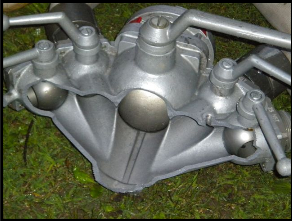
Figure 2 - Main portion of manifold after the failure.
