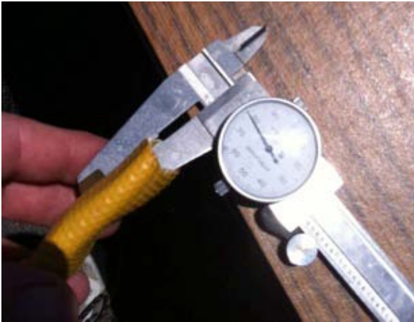
Avg. wall thickness times 2
