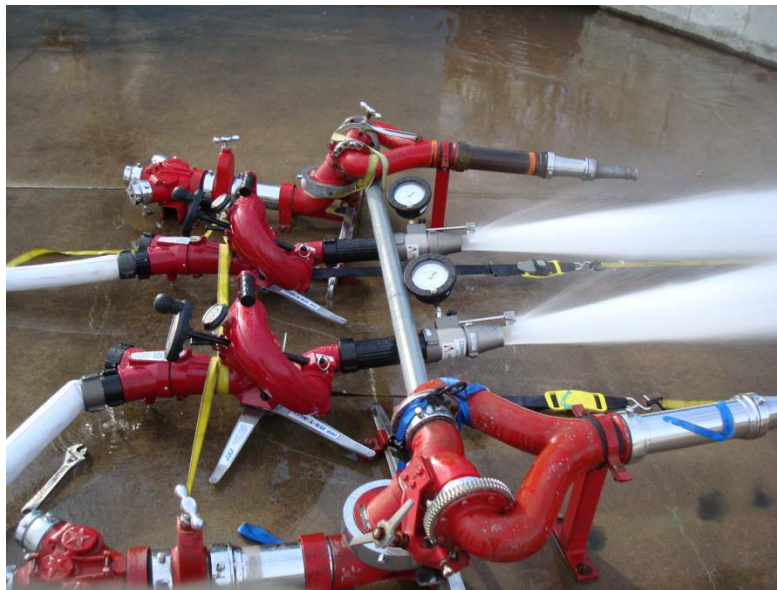
Figure 6. Multiple nozzle flow test at CONN
